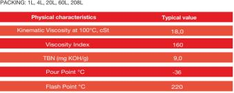
Top quality semisynthetic motor oil made with the use of a unique technology ACTIVE POWER, designed for four-stroke motorcycles and boats. ACTIVE POWER technology guarantees a low evaporation and fast starting. Reduces engine wear both at low and high temperatures, which helps extend the life of the motor and significantly reduces the fuel consumption. Ready to be mixed with other branded motor oils of this kind.
